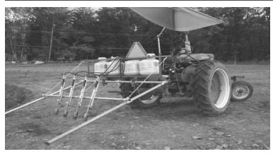
LP tanks are hooked up to four weed burners held about 8 in. off the ground.
