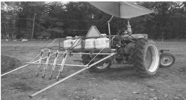
**LP tanks are hooked up to four weed burners held about 8 in. off the ground.**
