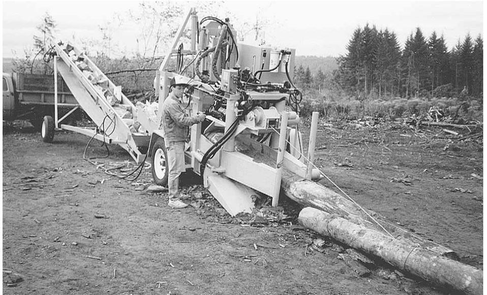
**A winch pulls log into chomper. Shear blade cuts 80% of the way through log and then drags log forward, pushing the end against a fixed set of splitting blades. Once the log is split, the shear completes its cut.**
