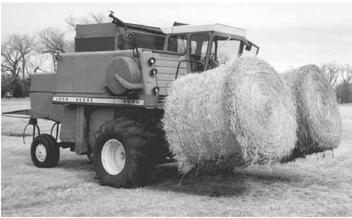
Chuck Misek wanted an easier way to move big round bales. So he converted an old Deere 6600 combine. It can move two bales at a time.
