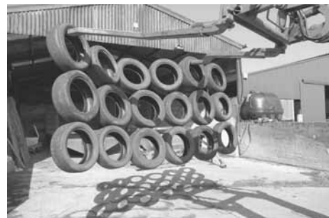
"It works much quicker than placing individual tires on a bunk silo," says Irish inventor Liam Murohy, who came up with a way to fasten tires together into large mats.
