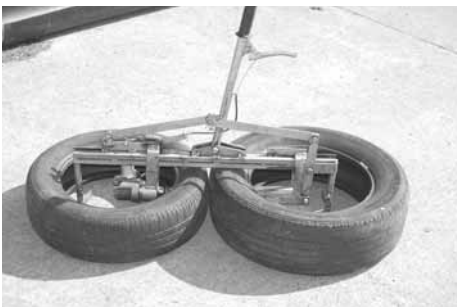
"It works much quicker than placing individual tires on a bunk silo," says Irish inventor Liam Murohy, who came up with a way to fasten tires together into large mats.
