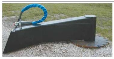
Hydraulicallypowered rotary tree saw fits skid loaders or can be 3-pt. mounted.
