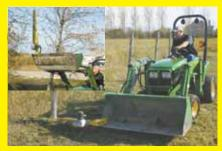
Hydraulic-powered cutter attaches to loader bucket.
