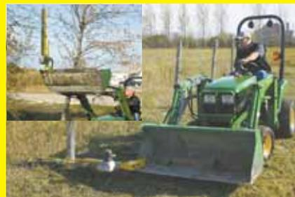
Hydraulic-powered cutter attaches to loader bucket.
