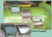
The Kuchar Helical Rasp Bar conversion kit greatly improves the thresh and capacity of STS combines 20 to 25% while reducing overall engine load and gives a much cleaner grain sample. These bars give the rotor more inertia for better fuel economy.
