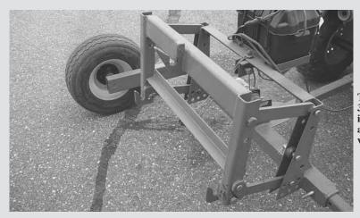
Tow-behind 3-pt. hitch is lifted by an electric winch.
