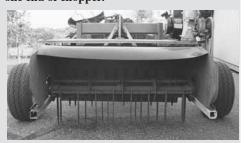
Engine belt-drives existing drive pulleys on chopper.
