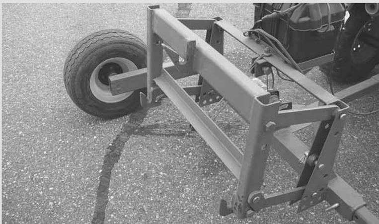
Tow-behind 3-pt. hitch is lifted by an electric winch.
