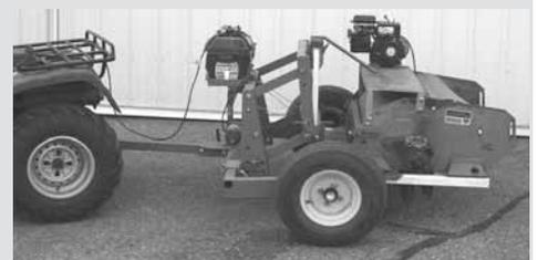
Power is supplied by a gas engine, mounted at one end of chopper.
