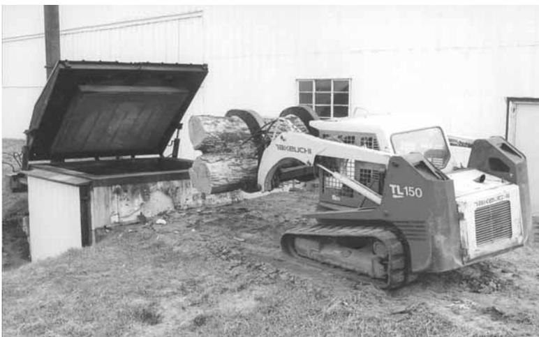
**They use a skid steer with a grapple to load up to three 6-ft. logs at a time.**
