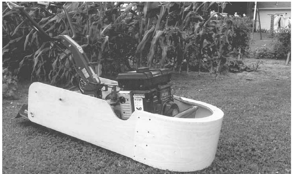
Caster wheel under front end follows garden terrain. Shroud can be removed quickly by pulling two bolts.
