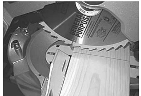
**Designed for chop, miter, abrasive, radial and hand power saws, the add-on laser guide turns on automatically only when the blade starts to rotate and shuts off when it stops.**
