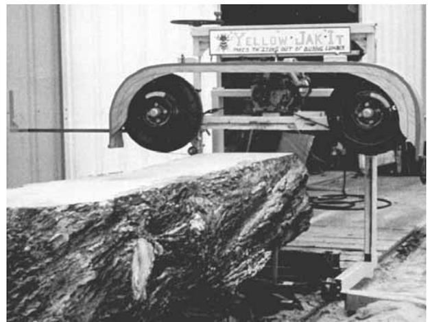
**Bill Reeks builds his bandsaw mills using two car wheels with the bandsaw blade wrapped around the outside of the tires. Tension on the blade is adjusted by adding air to the tires.**
