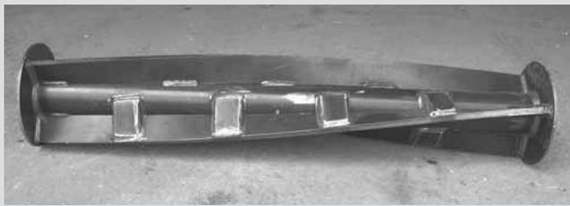
Rock beater has a spiral shape, which ensures that 70 percent of the opening in the beater is always open so crop can flow smoothly into rotor.
