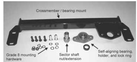
**Installation of stabilizer requires no drilling. It provides support to steering sector shaft and eliminates sector shaft play in steering box.**
