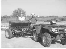
Kenneth Hill had friend Andy Fenley cut an old Minneapolis Moline 14-ft. end wheel drill in half to build this 6-ft. 8-in. wide drill. He pulls it with an ATV or small tractor.
