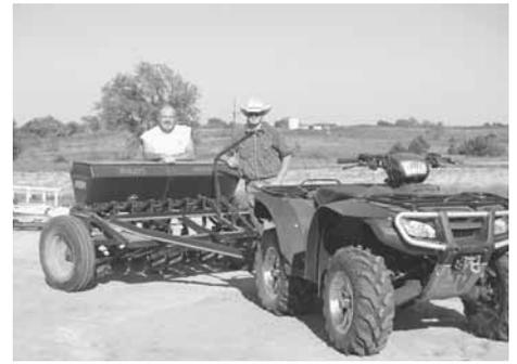
Kenneth Hill had friend Andy Fenley cut an old Minneapolis Moline 14-ft. end wheel drill in half to build this 6-ft. 8-in. wide drill. He pulls it with an ATV or small tractor.
