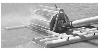
Water-driven, self-cleaning screen is designed to work in water as shallow as 4 in.
