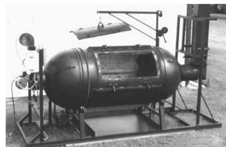
**Rotating Turn-A-Nator tumbles the carcass as it burns, using as little as 1/2 gal. of fuel per 100 lbs.**
