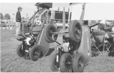
Photo shows 2-wheel-drive model, left, and 3-wheel-drive model, which is also fitted with optional rear wheel kit.
