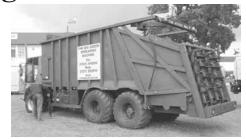
Four vertical spreader beaters mount on back of garbage truck. Truck's original hydraulic-operated ram pushes manure onto chain-driven slat floor in front of beaters.
