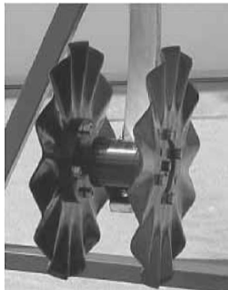
The Vertical Tillage Coulter Kit Attachment can be equipped with a wide selection of coulter blades. Spaced on 6-in. centers, the coulter blades can be matched to achieve the desired amount of tillage and residue sizing. **Patent Pending.**
