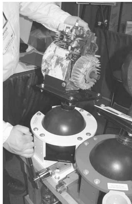
**Vise design allows you to work on all sides of an object without having to reclamp.**
