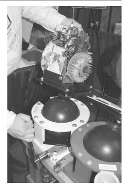
Vise design allows you to work on all sides of an object without having to reclamp.
