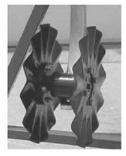
The Vertical Tillage Coulter Kit Attachment can be equipped with a wide selection of coulter blades. Spaced on 6-in. centers, the coulter blades can be matched to achieve the desired amout of tillage and residue sizing. *Patent Pending.*
