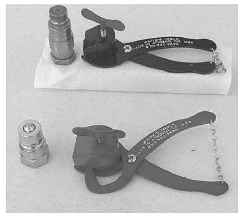
Tool works like pliers to grip the valve end. Turn a simple tap on one side of the pliers and it releases pressure as needed. “It works so smoothly you can release fluid into a Dixie cup,” says George Waite.
