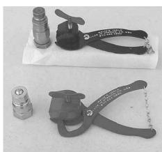
Tool works like pliers to grip the valve end. Turn a simple tap on one side of the pliers and it releases pressure as needed. "It works so smoothly you can release fluid into a Dixie cup," says George Waite.
