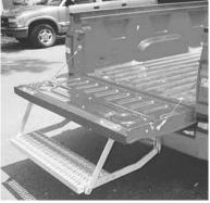
Add-on step bolts onto pickup's bumper and also onto back side of tailgate.
