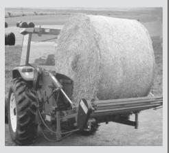
Bale shredder attaches to a 3-pt. hitch or quick-taches to a front-end loader.
