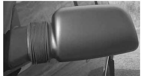
Extending mirror is electrically-operated, extending with the flip of a switch.
