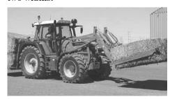
Depending on the model and the tractor/loader combination, an operator can pick up one to six bales at a time.
