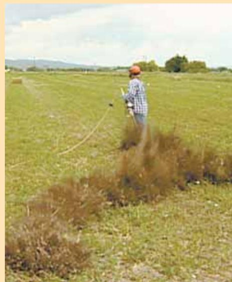
A mixture of oxygen and propane are injected underground and then ignited by the Rodenator to kill underground pests. You can see videos, photos and more information at the company's website: [www.rodenator.com](http://www.rodenator.com).
