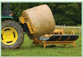
Bale feeder uses a bale unroller table that feeds hay out, and a set of 3-pt. bale spears that carry bale unroller around and also provide the hydraulics to power it.
