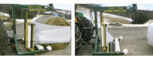
Once bale is wrapped, clamp arm cuts off the plastic and holds it for the next bale. A pair of angled rollers keep bale centered between the 2 arms.
