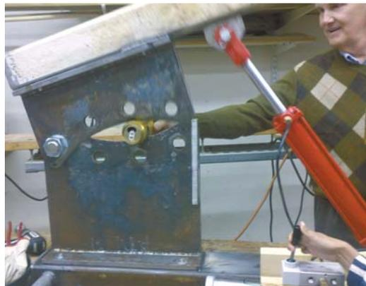
Retracting a hydraulic cylinder causes shears to slice cleanly through nearly anything, including nails.
