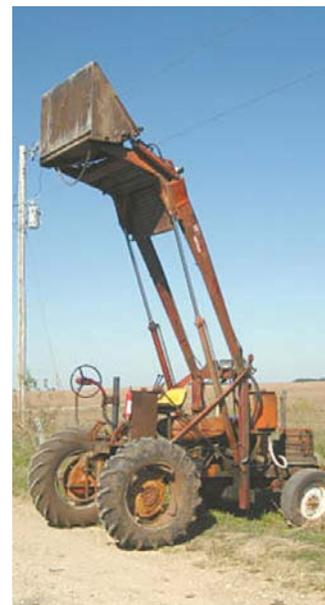
Loader on reversed AC WD45 tractor can lift 16 ft. high.
