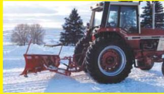
that would hold it at the right angle and also let me use the original 8-in. hydraulic cylinder. I also had a machine shop widen the blade 2 ft. on either side – from 7 ft. to 11 ft. – so the plow would move snow outside the wheels. Works like a charm. (Louie Waelti, Monroe, Wis.)
