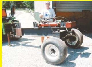
anything that it won't split. I used steel tubing to build the trailer's axles and bought new spindles and welded them in. It rides on 11.5 by 15 implement tires. A toolbox on back is used to store wedges. I already had the engine and most of the steel. The only items I bought were the pump and hydraulic hoses. I don't know exactly how much I spent to build it, but I know I saved a lot of money. (Larry Power, 16253 Snyder Rd., Petersburg, Ill. 61675 ph 217 632-3179)
