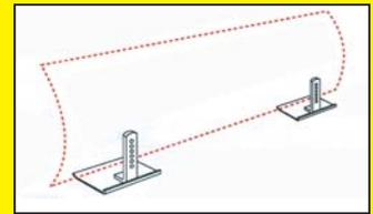
blade edge. They mount in existing skid shoe holes on the back side of the blade and can be adjusted for height using holes in the mounting bracket.
