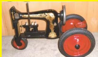
After reading a story in FARM SHOW on "sewing machine" tractors (Vol. 32, No. 2), I decided to make my own. It has a "motor" made from channel iron with chainsaw spark plugs; a radiator fashioned out of an old wood rasp; a chrome exhaust stack; and a seat made from a small electrical box. There's even a drawbar on back. The rear wheels are off a golf bag caddy, and the front wheels from a shopping cart.
