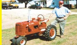
I had a lot of fun building this 1/2-scale Farmall Super M tractor. I started with a 1969 Cub Cadet 106 garden tractor equipped with a 12 hp Kohler engine and 3 flat tires and a rotted-out seat.
