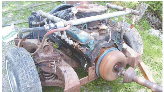
Dan Jamison converted the engine out of a late 1970's Cadillac into this powerful air compressor/sandblaster.
