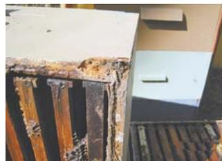
Fixit, a synthetic repair compound, was originally designed to repair damaged wood (left) in beehives and frames. It can be easily manipulated to hold form and shape.
