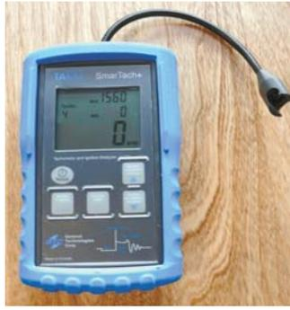
Wireless tachometer and engine analyzer makes troubleshooting and fine-tuning small engines an easier job.
