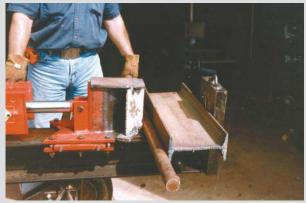
Photo shows Hochstetler straightening out a steel pipe. I-beam holds pipe in place.
