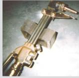
Attachment's pointed metal rod sticks out beyond torch's cutting head. It slides up and down torch, cutting neat holes up to 12 in. in dia.
