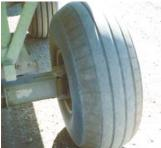
Rex Gogerty, Zearing, Iowa: "I have a gravity wagon with big flotation tires, and over the years the inside part of the tires wore out faster than the rest of the tires. The extra wear was so bad on one tire that I had to replace it. I know if I had rotated the tires they would have lasted longer. The tires should be cross switched front to back and left to right, and they should also be turned around."
