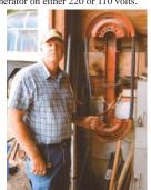
Tom De Clerck, Pana, Ill.: "I can store up to 200 ft. of air hose neatly out of the way with this homemade 'split wheel' holder. I cut a car wheel rim in half and welded a 4-ft. length of 4-in. channel iron to the back side of both rims. Then I bolted the channel iron to the wall. I just wind up the air hose in big loops on the rims. I mounted the unit near the door of my garage, where the air hose is readily available for any inside or outside
