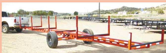
Irrigation pipe trailer rides on high-quality, all terrain tires. Model shown is designed to hold 40-ft. lengths of pipe.
