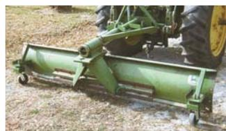
Add-on caster wheels keep blade from digging into ground.
