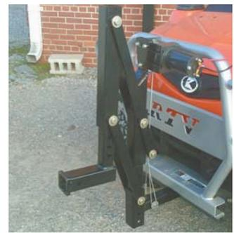
SwiftLift system fits into vehicle's 2-in. receiver hitch and accommodates 17 different attachments.
