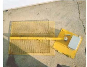
If safety gate is unlatched and swung open, the power shuts off to auger. Shutting the gate repowers the auger.
