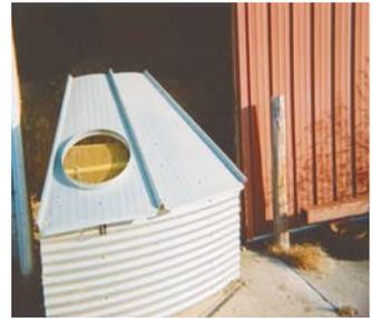
Safety latch makes it nearly impossible to run bin auger if someone is inside bin. It consists of an electric switch, a wire mesh guard gate, and an external latch.
