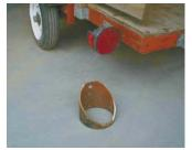
Protector is built from a short length of 6-in, dia, well casing, cross-cut at an angle.
