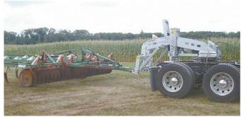
Fifth wheel boom turns a semi tractor into a wrecker/equipment mover, allowing you to quickly move farm equipment from one field to another.
