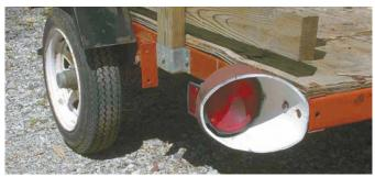
Andy Kozlowski built this "protector" out of old well casing pipe to protect the tail
