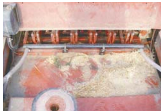
Plastic tubing runs back to nozzles directed at baler's knotters. The blast of air is controlled by electric solenoid valves connected to a switch in tractor cab.
