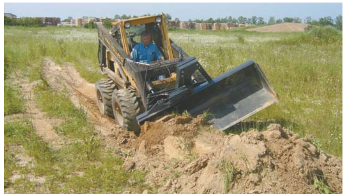
Tilting Bucket Hitch allows loader bucket to tilt up to 30 degrees, making it useful for digging ditches, cutting into side hills, etc.
