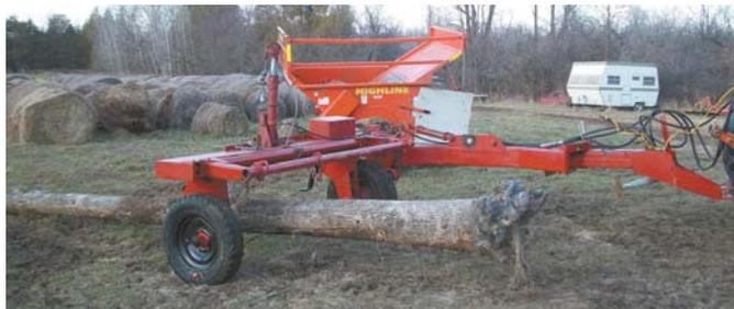
Doug Cook stripped an old mower-conditioner down to the frame, turning it into this low-cost log hauler. It can handle 18-in. dia. logs up to 20 ft. long.
