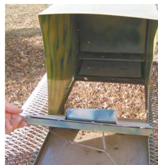
Bait is placed on trigger. When animal goes for the bait, it sets off the trigger and dumps animal into cage.
