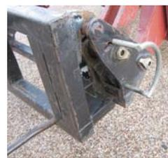
Cylinder is used to push and pull latch pins from the center, where it's less likely they'll get damaged or bent.
