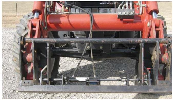
Quick-tach system latches and unlatches from the cab using a single hydraulic cylinder.
