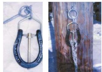
EZ-Tie hitch consists of a horseshoe with a swivel-type drawbar pin, and a clevis that attaches to pin handle. Pin swings back out of the way to make room for lead line.
