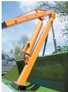
He removed the legs and wheels from the hoist, keeping the ram and lift arm intact.
