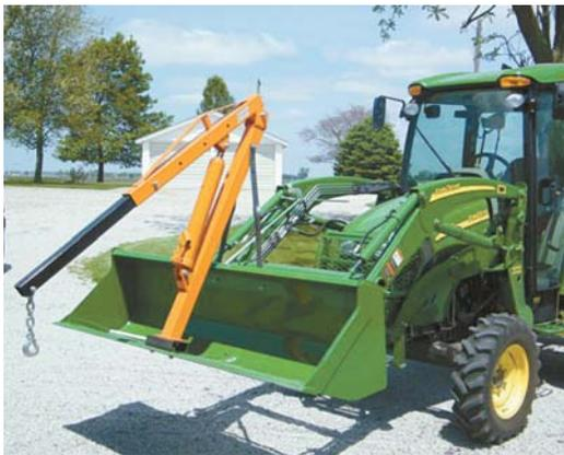
Tom Roland mounted an engine hoist on his loader bucket, boosting its lift height to almost 18 ft.
