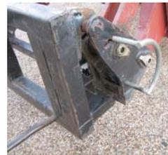
Cylinder is used to push and pull latch pins from the center, where it's less likely they'll get damaged or bent.
