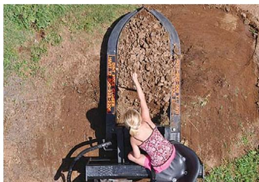
There’s a platform behind the dozer blade where someone can hold a bare root tree or fence post steady as the hole is being filled.
