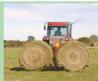
Two Banger bale accumulator picks up 2 bales, one on either side of tractor (far left). Once loaded, wings on either side of rear-mount bar swing backwards so paired bales can then be carried off the field or down the road
