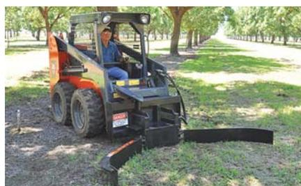
Skid loader-mounted “dirt hole closer” has a pair of 60-in. long, 10-in. high steel wings that open up 8 ft. wide.
