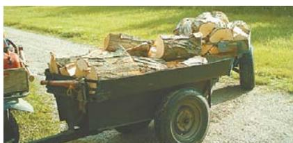
**ATV-pulled trailers are designed to haul logs one behind the other. Both trailers were made from a single 200-gal. fuel oil tank.**
